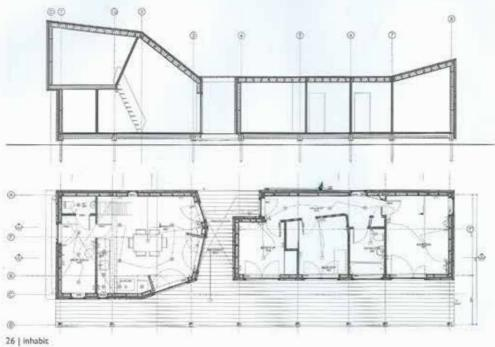
north wall provides privacy and insulation, while the house remains very open to the south where a large veranda acts as an extension of the living space. The roof form is generated by the need to gain maximum east sunlight penetration into the master bedroom at one end, and to provide a first-floor living space with high natural surveillance over the campus at the other.  $\Box$
