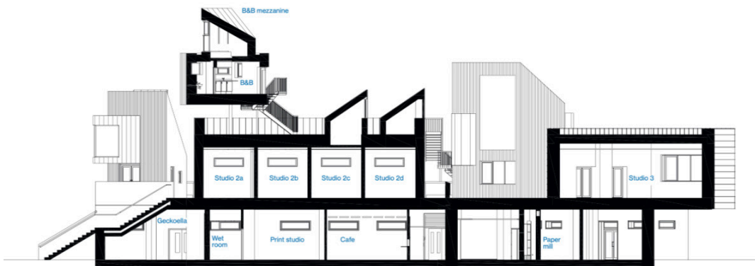
Above: Section through the northernmost wing showing external staircase giving public access to the first-floor studios and a cross section through one of five rooftop accommodation pods.
